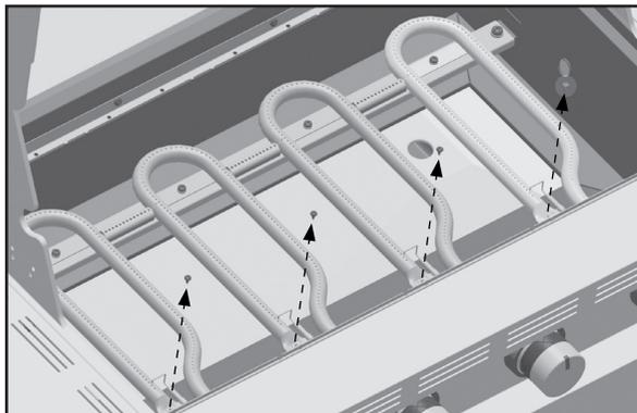
Remove the self-tapping screw from each electrode as shown in **Figure 2**.
