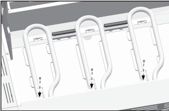
Use the new self-tapping screws to secure the electrode to the new double burner as shown in **Figure 6**.
