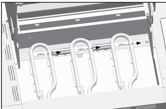
Remove the hitch pins from the double burners and carryover bar as shown in **Figure 2**.
