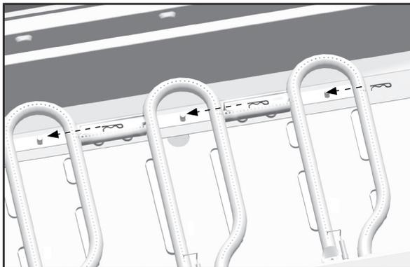
Use the new hitch pin to secure the new double burner to the carryover bar as shown in **Figure 5**.
