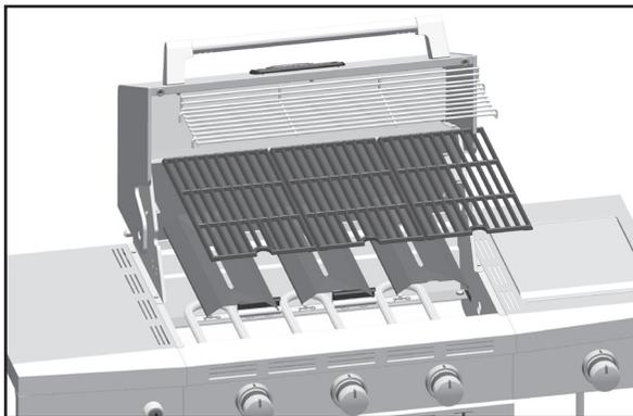
Lift the top lid. Remove the cooking grates and flame tamers to reveal the double burners.
