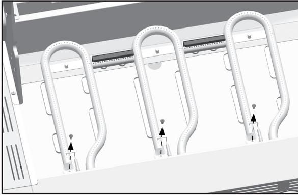
Remove the self-tapping screw from each electrode as shown in **Figure 3**.
