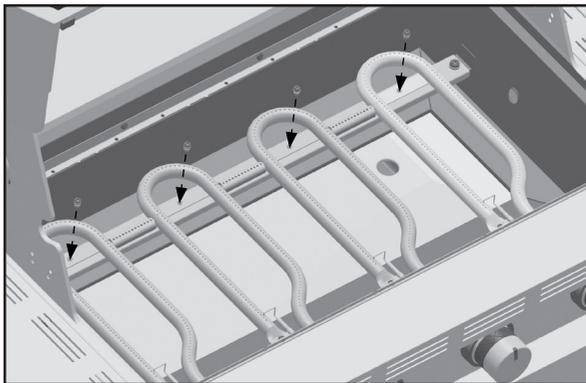
Use the new hardware to secure the new double burner to the carryover bar as shown in **Figure 6**.
