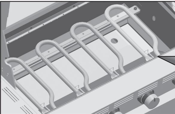
Replace the old burner with the new double burner. Ensure that the venturi is seated correctly over the valve **Figure 4**.
