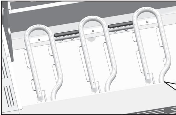
Replace the old burner with the new double burner. Ensure that the venturi is seated correctly over the valve **Figure 4**.
