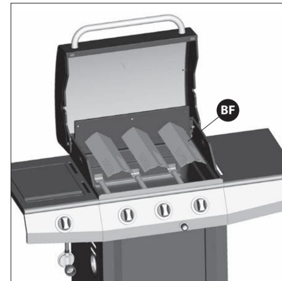
First place the flame tamers (BF) and then the cooking grates (BG) into the burner box.
