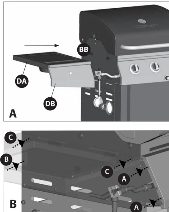
**TIP:** To position the left side burner shelf, insert the two hooks on the side shelf assembly into the support brackets located on the upper left side panel (BB).
