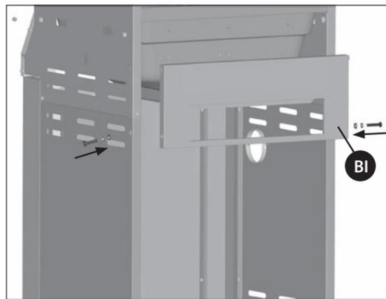
Attach the upper back panel (BI) to both the left and right side panels (DE and DF).
