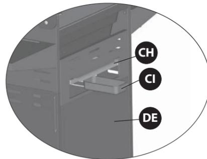
a. Insert the grease tray (CH) into the opening in the upper back panel (BI), making sure to engage tracks located under burner box.
