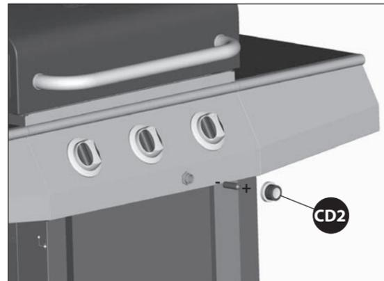
Unscrew the electronic igniter button (CD2) and insert one AA battery into the electronic igniter battery compartment, with the positive end facing outward.
