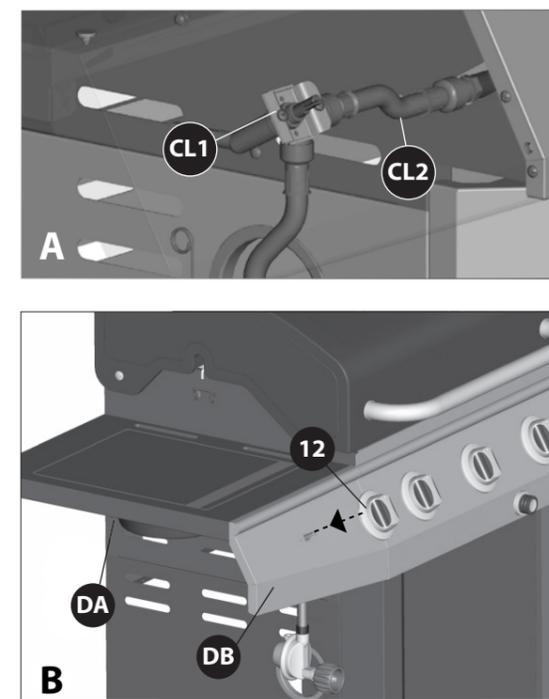
Remove the hardware that is pre-assembled to the side burner valve bracket (CL1), as shown in figure B. Insert the side burner valve stem through the rear of the left side shelf fascia (DB). Assemble the side burner valve (CL1) to the side shelf fascia (DB), using the hardware removed.
