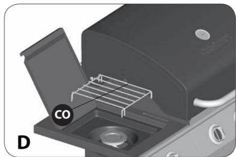
d. Place the side burner cooking grate (CO) into position on the side burner shelf, as shown in figure E.
