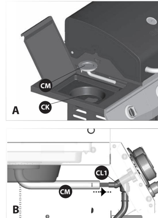
a. Position the side burner (CM) through the opening in the left side burner drip pan (CK).
