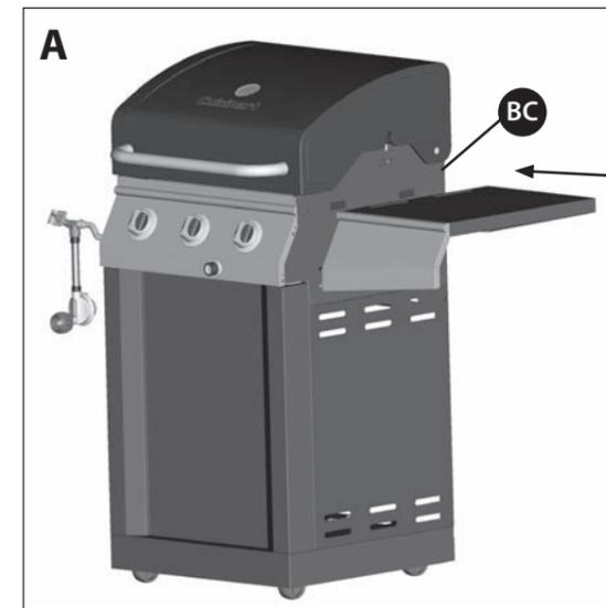
**TIP:** To position the side shelf, insert the two hooks on the right side shelf assembly into the support brackets located on the upper right side panel (BC).
