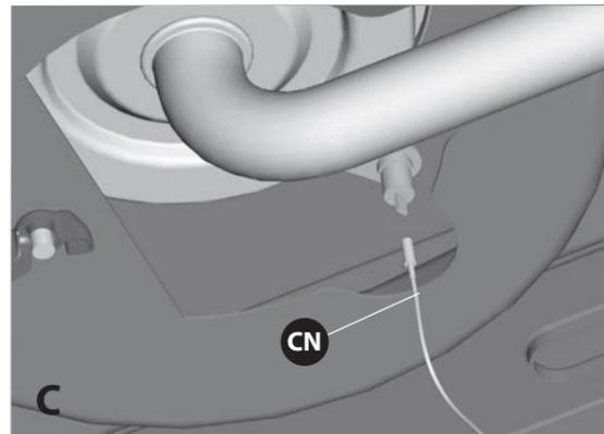
c. Attach the end of the side burner electrode wire (CN) to the underside of the side burner electrode, as shown in figure D.
