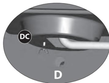
d. Using the wing nut provided, assemble the side burner to the side burner drip pan (DC), as shown in figure D.
