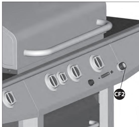
Unscrew the electronic ignitor button (CF2) and insert one AA battery into the electronic igniter battery compartment, with the positive end facing outward.
