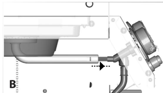
b. Make sure that the side burner (DD) engages the side burner valve (CC) as shown in figure B.
