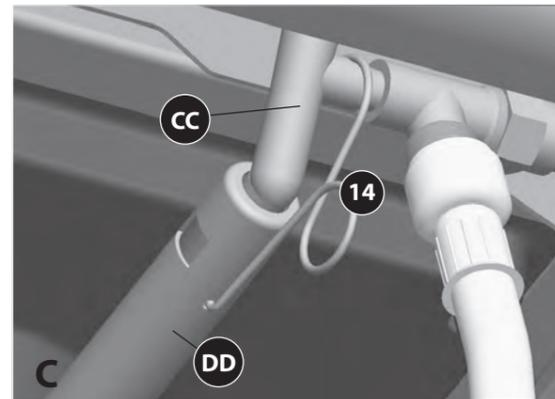
c. Use the side burner Venturi clip (#14) to connect the side burner (DD) to the side burner valve (CC).
