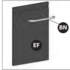
a. Assemble the towel bar (BN) onto door (EF).
