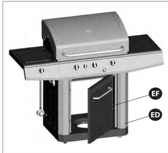
b. Hold the door perpendicular to the BBQ Cart. Align the two clasps on the door hinge (EF), with the two holes on the right side pillar (ED). Once aligned push the two clasps into the openings, and immediately push down to lock clasps in place.
