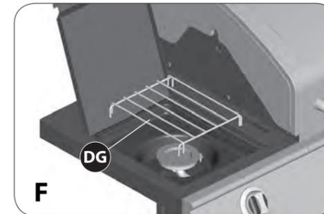
f. Place the side burner cooking grate (DG) into position on the side burner shelf, as shown in figure F.
