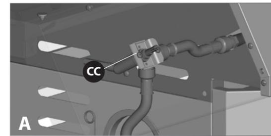
Remove the hardware that is pre-assembled to the side burner valve bracket (CC), as shown in figure A. Insert the side burner valve stem through the rear of the left side shelf fascia (DB). Assemble the side burner valve (CC) to the side shelf fascia (DB), using the hardware removed.
