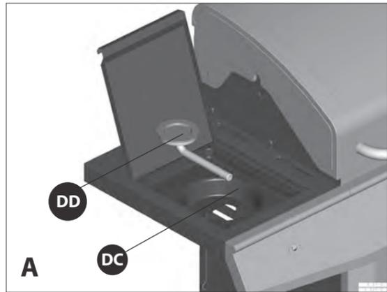
a. Position the side burner (DD) through the opening in the left side burner drip pan (DC).
