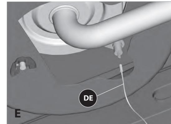
e. Attach the end of the side burner electrode wire (DE) to the underside of the side burner electrode, as shown in figure E.
