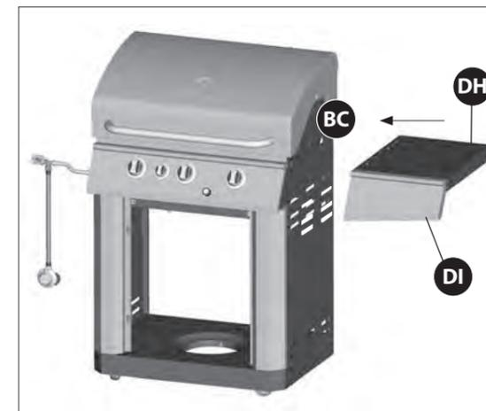
**TIP:** To position the right side shelf, insert the two hooks on the side shelf assembly into the two support brackets located on the right upper side panel (BC).
