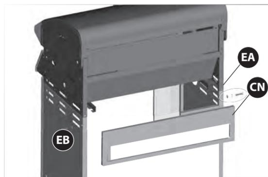
Attach the upper back panel (CN) to both the left and right side panels (EA and EB).
