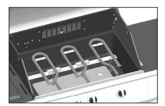
Use the new self-tapping screws to secure the electrode to the new double burner as shown in **figure 5**.
