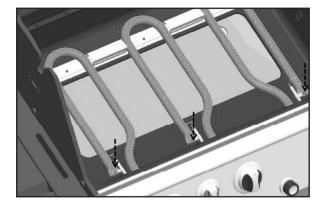
Place the new double burners into the burner box. Ensure that the venturi is seated correctly over the valve **figure 4**.
