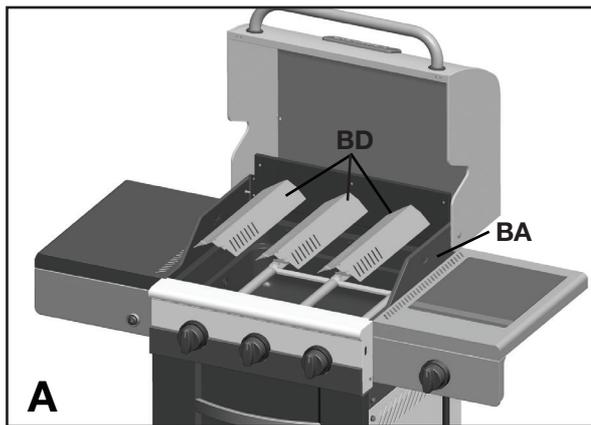
a. Place the Flame Tamers (BD) into the Burner Box (BA).
