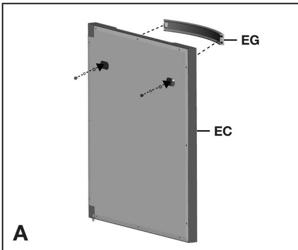
Assemble the Door Handle (EG) to the Door Assembly (EC) as shown in Figure A.
