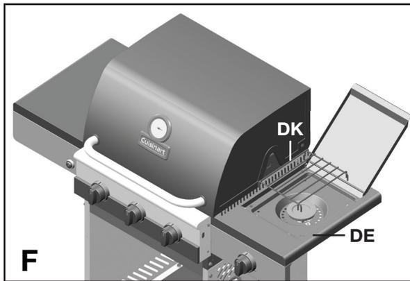
e. Place the Side Burner Cooking Grate (DK) into position on the Side Shelf (DE), as shown in figure F.
