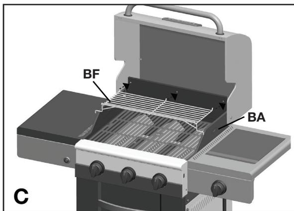
c. Place Warming Rack (BF) onto the Burner Box (BA) by inserting the three positioning rods into the rear panel of the Burner Box (BA), as shown.
