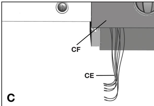
**TIP:** The Electrode Set, Main Burner (CE) wires can be found attached to the Control Panel heat shield (CF), as shown.
