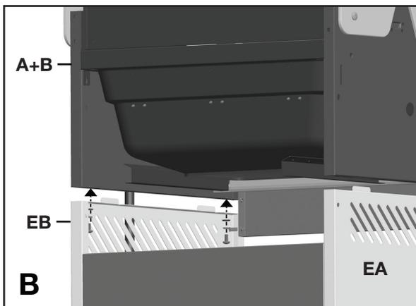
b. Assemble the Burner Box Assembly (A+B) to the Left and Right Cart Side Panels (EA + EB), as shown.
