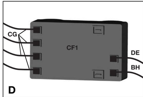
e. Insert the Electrode Wire, Infrared Zone (DE) and the Electrode Wire, Rotisserie Burner (BH) into the Electronic Ignition Assembly (CF1), as shown in figure E.
