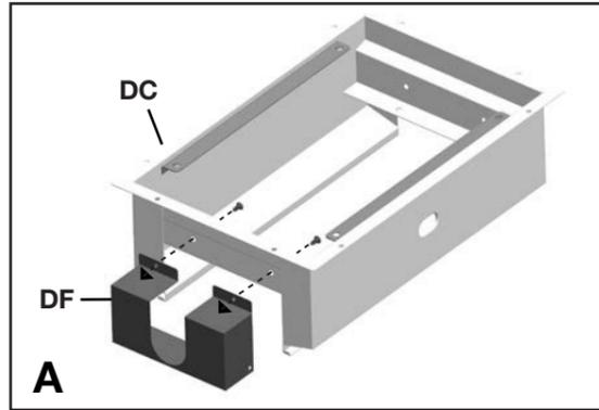
a. Assemble the Infrared Side Burner Wind Shield (DF) to the Infrared Support Frame (DC), as shown in figure A.
