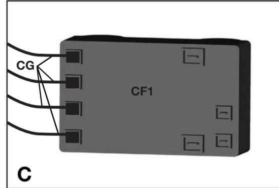
d. Insert the four Electrode Set, Main Burner wires (CG) into the Electronic Ignition Assembly (CF1), as shown in figure D.
