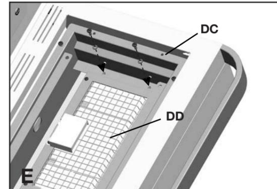
e. Assemble the Infrared Zone Side Burner (DD) to the Infrared Zone Support Frame (DC), at the 2 points indicated in figure E.
