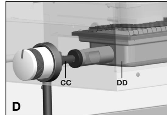
d. Make sure that the Infrared Zone Side Burner (DD) engages the Side Burner Valve (CC) gas jet, as shown in figure D.
