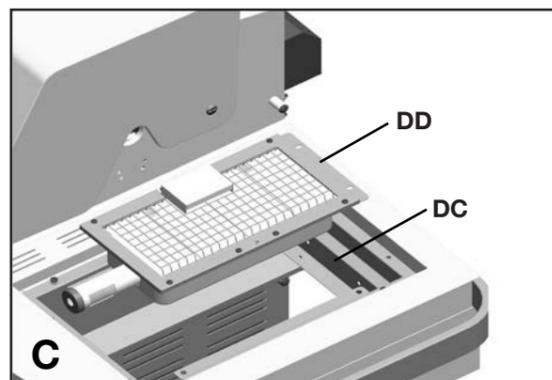
c. Position the Infrared Zone Side Burner (DD) through the opening in the Infrared Support Frame (DC).
