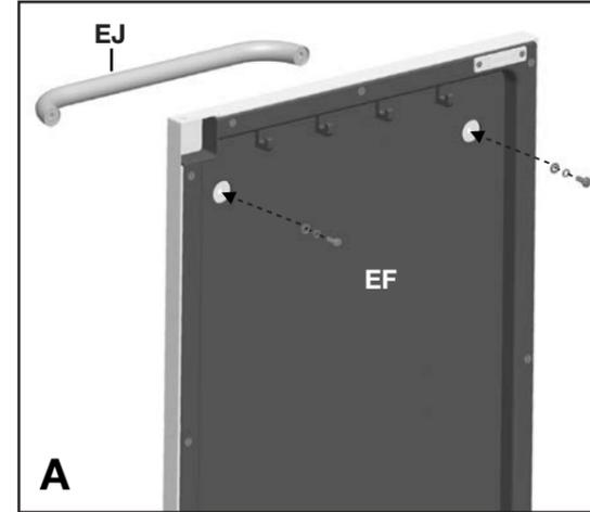
Assemble the Door Handle (EJ) to the Left and Right Door Assembly (EF and EH) as shown in figure A.
