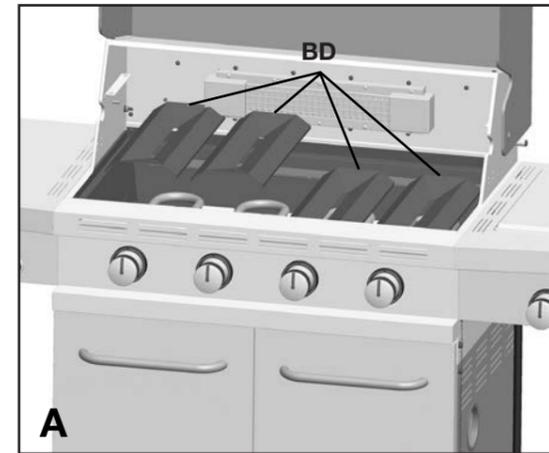
a. Place the Flame Tamers (BD) into the Burner Box Assembly (BA).
