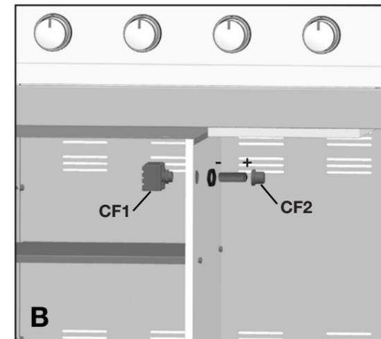
a. Remove the Electronic Ignition Battery Cap (CF2) and the plastic nut from the Electronic Ignition Assembly (CF1) and feed the Electronic Ignition Assembly (CF1) through the opening in the Interior Cart Divider (CQ), and secure using the nut.
