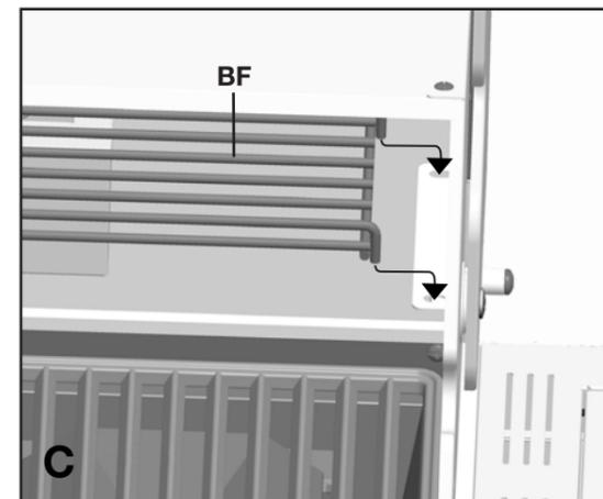
c. Assemble the Warming Rack (BF) by inserting the fixed pins into the warming rack support bars located on the Burner Box Assembly (BA), as shown.
