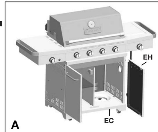
a. Assemble the Right Door Assembly (EH), to the Bottom Shelf (EC) by inserting the fixed pin (bottom of door) into the hole provided (figure B).
