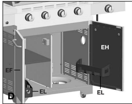
b. Assemble the top of the Right Door Assembly (EH) to the Front Brace (CK), by pressing in the door support pin and aligning with the hole located on the top right corner of the door.
