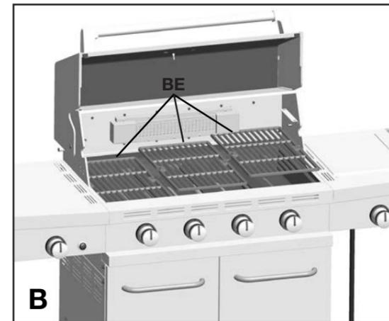
b. Place the Cooking Grates (BE) into the Burner Box Assembly (BA), as shown.
