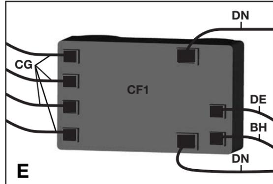
f. Insert the two Electronic Ignition Button (DN) wires into the Electronic Ignition Assembly (CF1), as shown in figure F.
